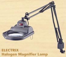
Energy-saving, 100w quartz halogen bulb with HI/LO position switch, produces 900' candles of illumination, with a scientifically-designed parabolic reflector. Full 5" diameter, 3-diopter glass lens. This task lamp has a 45" suspension reach. Includes architect's adjustable clamp with 21/2" opening, plus a convenience outlet in the base. Built-in handle on the shade. 9', 3-conductor grounded cord. Board attachment clamp included.
